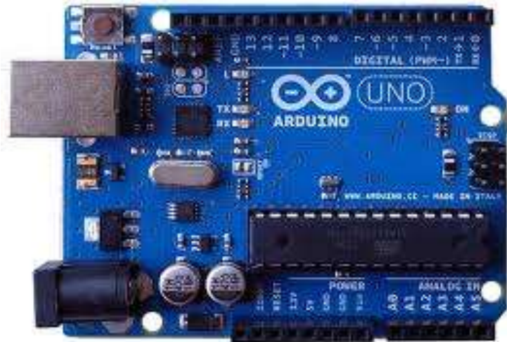
Gambar II.1 Board Arduino Sumber : Abdul Kadir : 2013 Hal 16
