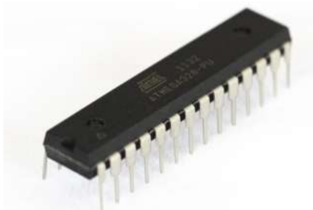
Gambar II.2 Mikrokontroler ATmega328 (Sumber: http://www.protostack.com )
