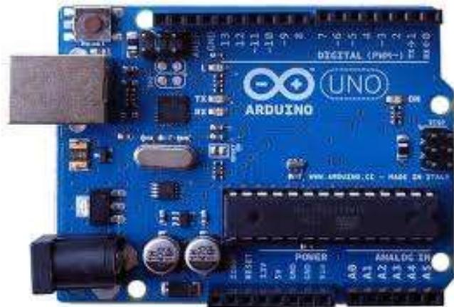
**Gambar II.2 Board Arduino**
