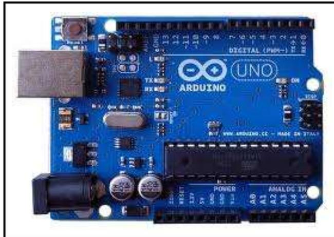
**Gambar II.2 Board Arduino**
