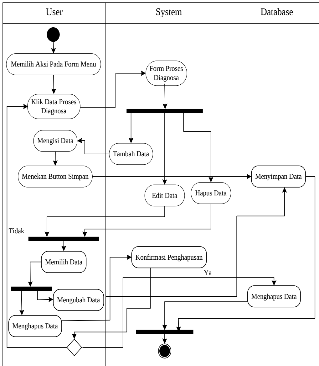
Gambar III.4. Activity Diagram Proses Diagnosa
