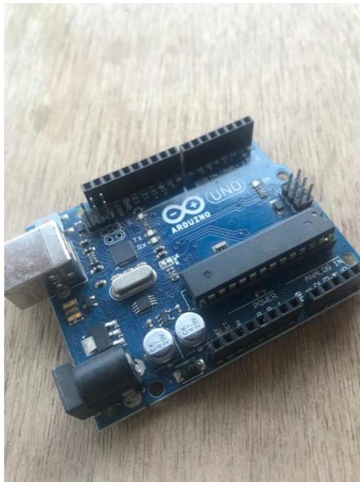
**Gambar IV.1. Development Board Arduino Uno**
