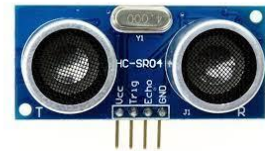
Gambar II.3. Sensor Ultrasonic HC-SR04
