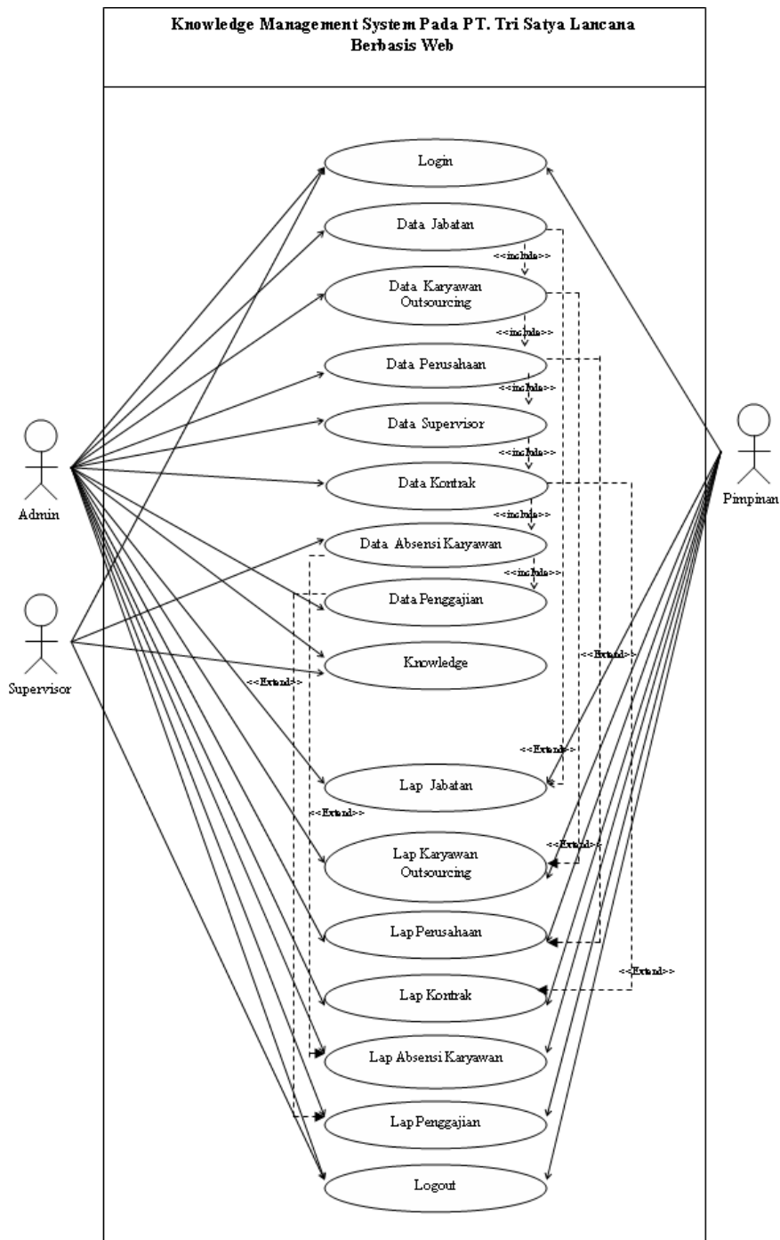
Gambar III.1. Use Case Diagram Knowledge Management System Pada PT. Tri Satya Lancana Berbasis Web
