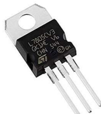
Gambar II.4 Ic Regulator 7805
