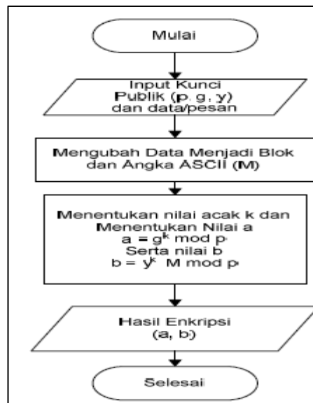
Gambar II.6 Flowchart Enkripsi Algoritma El Gamal
