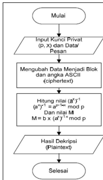
Gambar II.9 Flowchart Dekripsi Algoritma El Gamal
