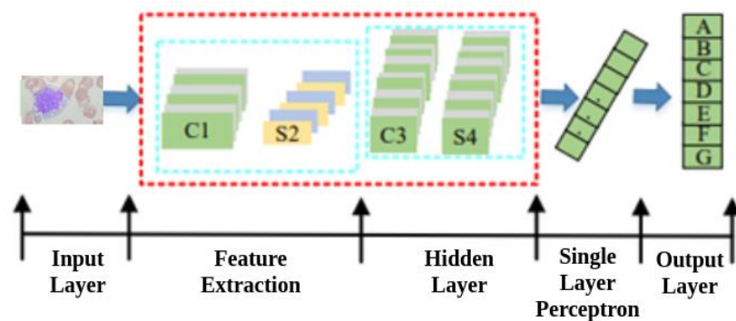
Gambar II.2 Struktur Convolutional Neural Network
