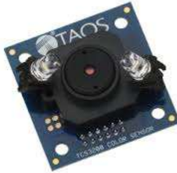
Gambar II.8. Sensor TCS 3200D
