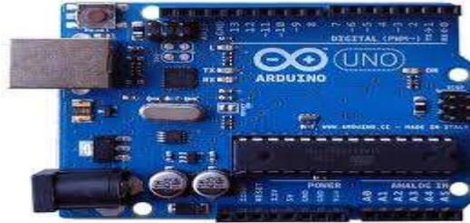
**Gambar II.3. Board Arduino**
