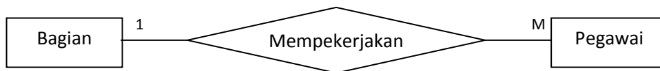
Gambar II.3 Contoh Pemetaan kardinalitas One to Many/ Many to One (Sumber : D. Tri Octafian ; 2011 : 151-152)
